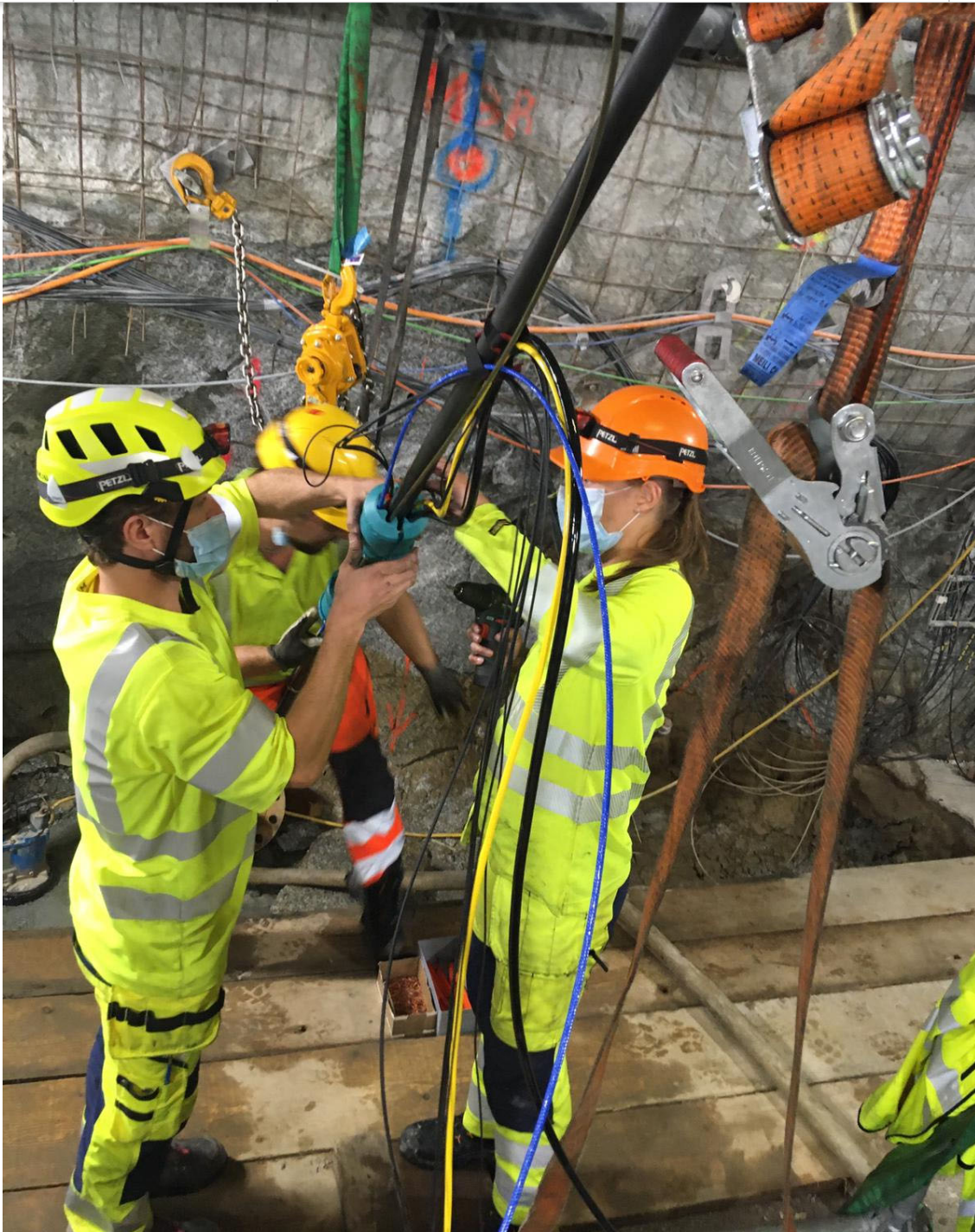
PhD student Kathrin Behnen (right) and Kai Bröker (left) installing the sparker in the borehole. © BedrettoLab, 2022
